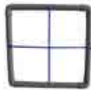
Figure 27: PVC Quadra subdivided into four 20 cm squares
