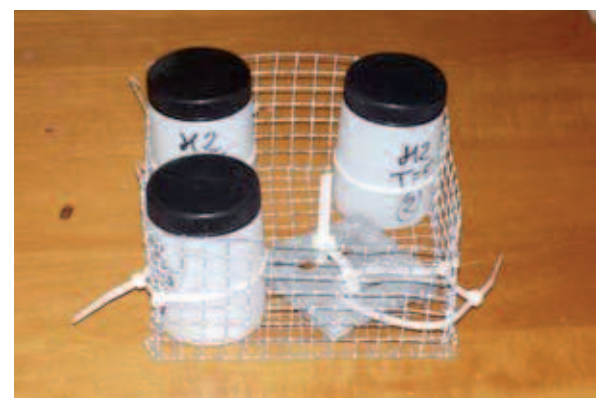
Figure 7 : Sediment trap with cylindrical PVC collector
