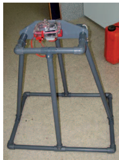
Picture 6: Rigid PVC reinforcement to be used for the photographic study (according to Garcia-Charton)
